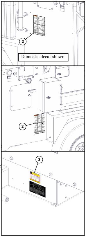
BC1200XL - Top of right side fender Domestic version shown BC1500 - Left corner of frame above serial tag BC1800XL - Left front corner of frame beside serial tag
