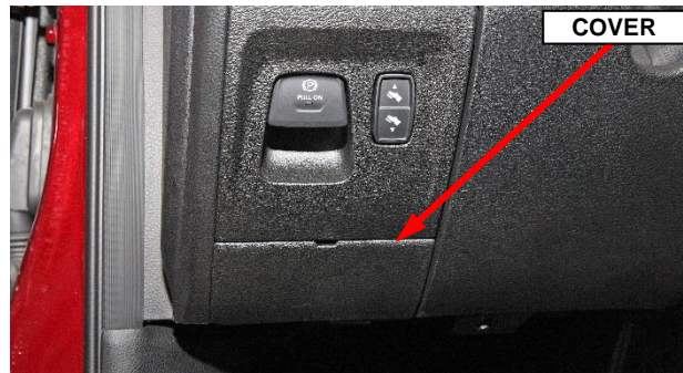
Figure 1 – Park Release Access Cover
