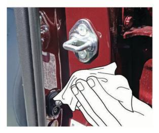
6. Apply the new certification label in the same location as the old label. Make sure the label is applied in the same orientation as the removed label.
