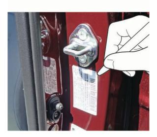
5. After the label is removed, using isopropyl alcohol on a lint-free cloth, thoroughly clean the area where the new label will be attached. Make sure there is no residue from the old label, and allow the alcohol to dry.
