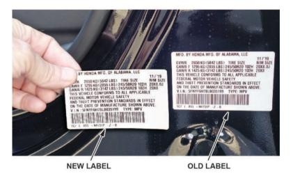
4. Use a plastic tool to remove the label. Be careful not to scratch or damage the paint.
