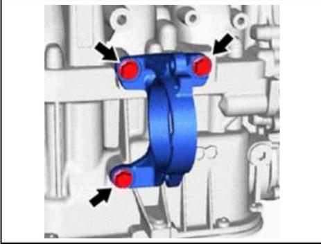
**6. TRANSFER DRIVE SHAFT BEARING BRACKET**
