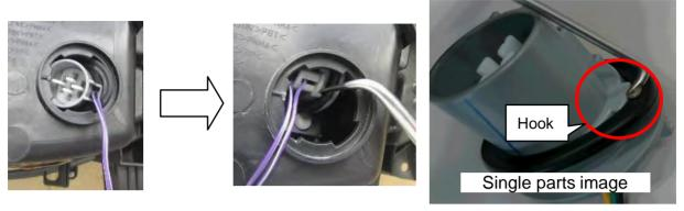
Note: Connector A will not drop down far enough to turn 90 degrees. This O ring has limited room and visibility. Watch Video A
