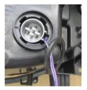
8. Push the O ring gasket into the four hooks at the bottom of the connector.
