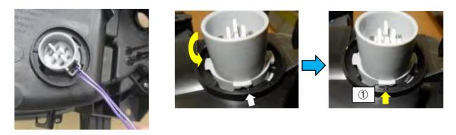
1 OK: Fits on rib protrusion.
