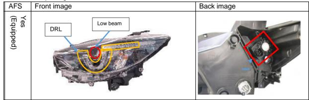
AFS: Adaptive Front Lighting system which enhances the range of visibility when the headlights are turned on by pointing the optical axis of the headlights in the direction in which the vehicle is advancing according to the steering operation. The swivel actuator constantly detects the headlight swivel angle from the hall sensor built into the actuator and inputs the swivel angle to the AFS control module via LIN communication.
