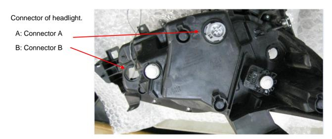
Caution: Be careful not to damage the headlight lens (scratch etc...) or deform the terminal.
