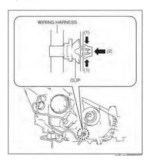
4. To prevent scratches or damage, affix protective tape to the position shown in the figure.
