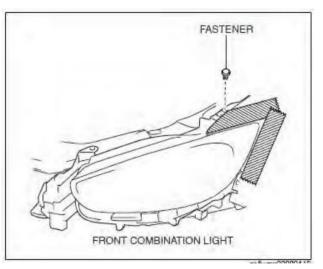
6. Pull the front combination light in the direction of the arrow shown in the figure and pull out the front combination light pin from the body.
