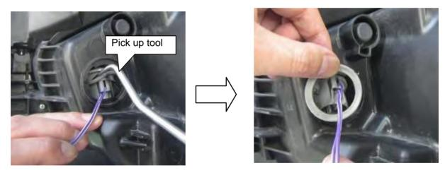
7. Install the gasket with new one (black one). Thread the new gasket onto the spare wire or string.
