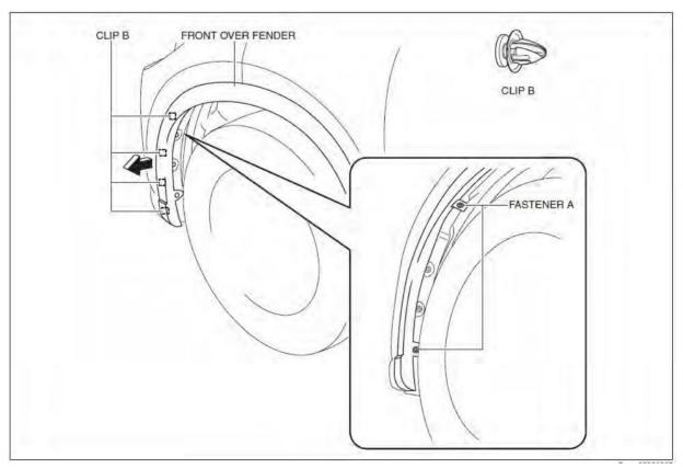
Pull the front over fender in the direction of the arrow shown in the figure, set the front over fender out of the way while detaching clips B.
