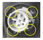
3. Install the gasket with new one (black one). Thread the new gasket onto the spare wire or string.
