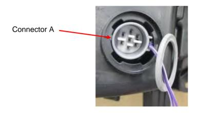
2. Replace the gaskets with the new black supplied gaskets of connector A and connector B and install the two gas absorption sheets.
