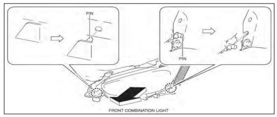
7. Remove the front combination light and proceed to Step D. Gasket replacement procedure.
