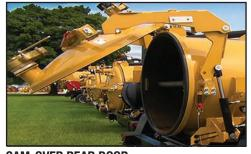
**CAM-OVER REAR DOOR.** Provides a 360-degree positive seal, even under reverse pressure without additional clamping requirements. The highly reliable cam-over door has a no in-tank moving parts, so all maintenance is external.
