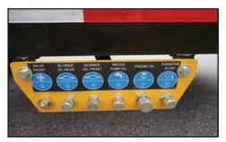
**REMOTE DRAINS.** Remote fluid drains and grease points are centrally located near operator controls for ease of service.
