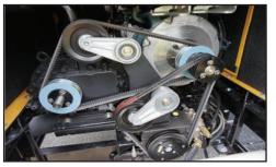
AUTO BELT TENSIONERS. Keeps proper belt tensions at all times and extends belt life.
