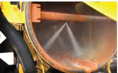
**IN-TANK WASH-DOWN.** Delivers a highpressure water spray to the tank interior helping simultaneously dump material and clean the inside of the tank. Saves clean up time and makes it easier to remove difficult debris.
