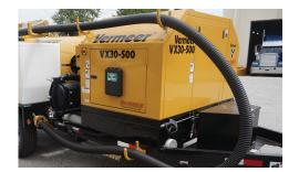
**NO HASSLE HOSE.** Hang the suction hose on the side of the machine when moving between jobsites instead of coiling or disconnecting it, increasing productivity and reducing operator fatigue.
