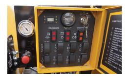
**LOCKABLE CONTROL PANEL.** All machine controls and gauges are secured and out of the elements.
