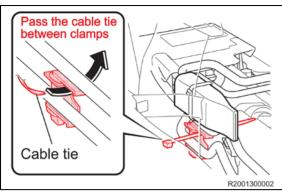
(6) Pass the cable tie between clamps.
