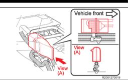
(7) Place the link connector on the instrument panel wire of the left side.
