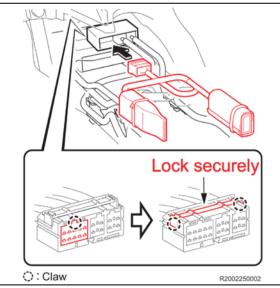
h) Connect the connector (30P) of airbag sub harness to the connector holder of the airbag sensor and lock the retainer securely.
