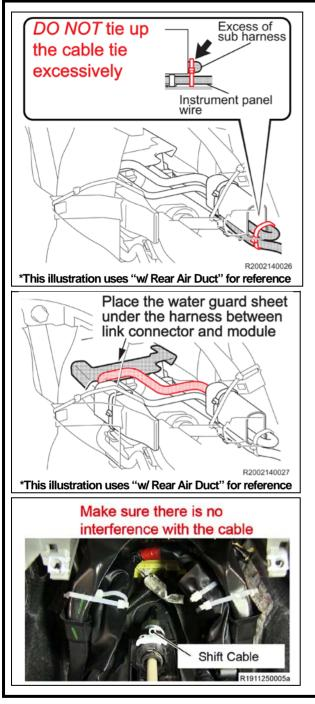
I) Using a cable tie, fix the excess harness of module side together with the instrument panel wire.
