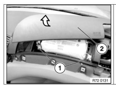
• Undo the screws (1) and place the front passenger's airbag cover (2) on top.
