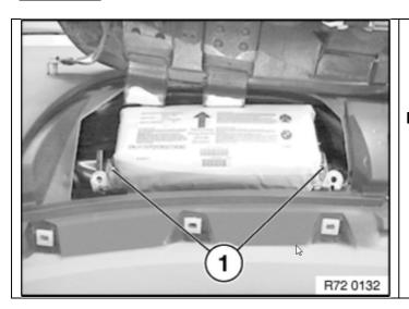
Undo the screws (1) at the front passenger's airbag module.
