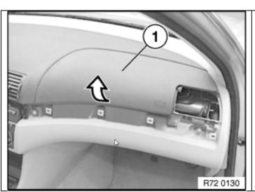
Lever out the front passenger's airbag cover (1).
