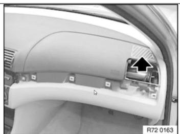
• Position of the retaining clip of the front passenger's airbag cover
