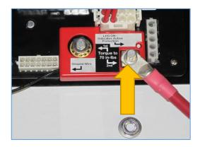
(2.4) Install power cable onto G9 Protection Module stud with conical washer nut and torque to 70 in/lbs.
