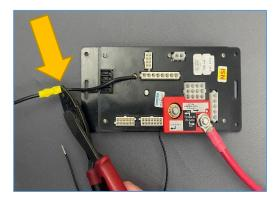
(2.5) Locate existing G9 ground wire connection and disconnect or cut wire.
