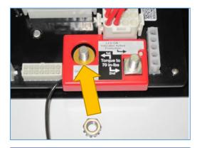
(2.3) Attach G9 Protection Module onto the G9 Power Stud with external tooth washer nut and torque to 70 in/lbs.
