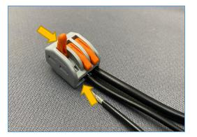
(2.6a) Splice G9 Protection Module ground wire to the existing G9 ECM ground wire. Strip each ground wire 10mm, insert each wire fully into Wago 222-413 terminal block, move orange tab from the open to fully locked position.
