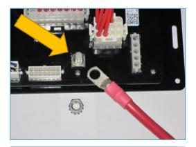
(2.2) Remove the external tooth washer nut and existing power cable from the G9 ECM power input stud.
