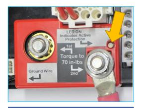
(2.7) Turn on Main Power Switch and verify that the LED illuminates.
