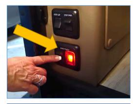
(2.1) Power off system by turning the Main Power Switch to the off position (located just inside the entry door).
