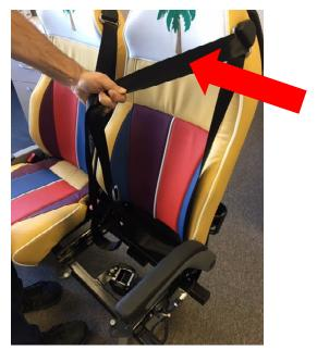
3.4. Remove belt retractor from chassis and dispose of hardware.
