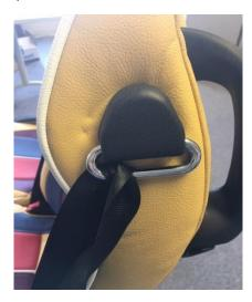
3.1.1.4. Remove seat cushion by lifting at front. Inspect webbing at retractor for rolling. Unroll webbing if this has occurred.
