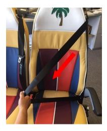
3.1.1.2. Inspect webbing for fraying, tears or wear. If conditions are present, retractor requires replacement.
