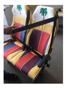
3.1.1.6. Release and allow webbing to feed completely back into retractor. Webbing return results in mechanism switching back to ELR functionality.
