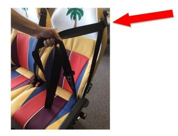
3.1.1.5. Retractor mechanism must switch to ALR functionality for child seat securement. Belt now works as a ratchet and webbing will ONLY feed in, not out.
