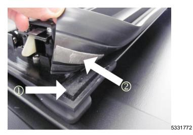
5. Locate the double-sided tape at both outer ends of the new seal. Remove the protective film and press the seal (2) firmly onto the corner cap (1), apply pressure for 15 seconds to allow the adhesive to bond. Perform this step on both ends of the new seal.
