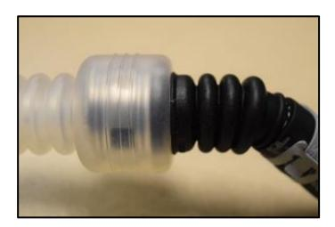
• When correctly seated, the fuel line coupling cover should appear as shown.
