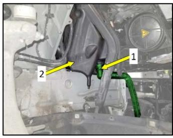
Connect secondary air hose <1> to air filter housing <2> if not previously done.
