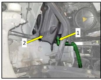
Disconnect secondary air hose <1> from air filter housing <2>.
