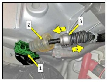
• Remove fuel line clip <1> using pry lever -80-200- (or equivalent).
