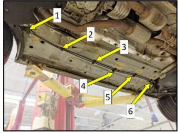
Install new fuel line clips <1 through 6>.
