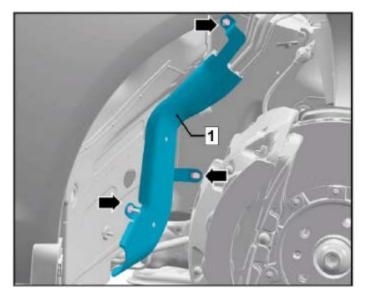
Remove nuts <arrows> and remove fuel line shield <1>.
