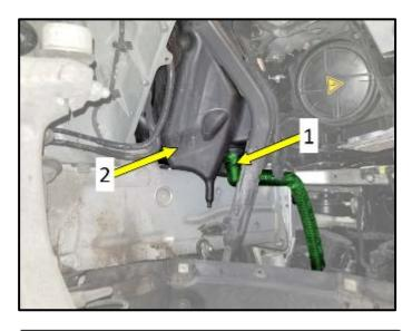
• Connect secondary air hose <1> to air filter housing <2> if not previously done.
