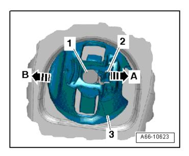
To remove the clips <3>, unlock the release lever <2> with needle nose pliers in direction of <arrow A> and push it off the pin <1> in direction of <arrow B>.
