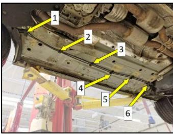
Starting at the front of the vehicle, remove fuel line clips in the order <1 through 6> using Pry lever -80-200- (or equivalent).
