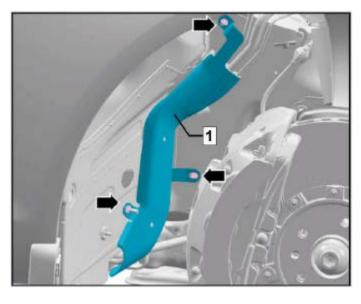
Remove nuts <arrows> and remove fuel line shield <1>.
