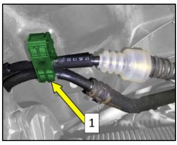
Remove fuel line clip <1> using pry lever -80-200- (or equivalent).
