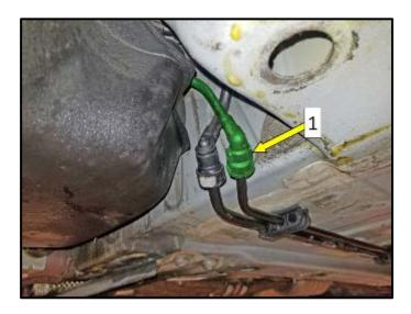
Remove the protective cap from the new fuel line and connect fuel line coupling <1> until it audibly engages.
