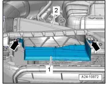
• Remove the bolts <arrows> and the air guide <2>.
