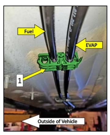
Note the orientation of fuel line, EVAP line and fuel line clips <1>.
