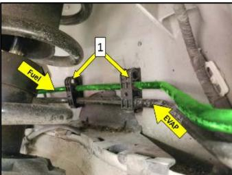
Remove the fuel line clips <1> using Pry lever -80-200- (or equivalent).
