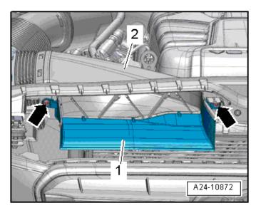
Install the air guide <2> and torque bolts <arrows> to 1.5 Nm.
