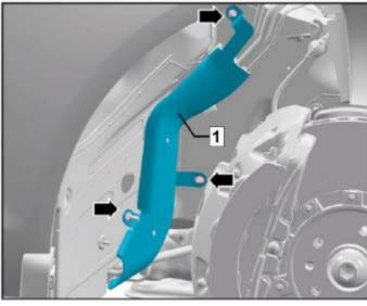
Install fuel line shield <1> and nuts <arrows>.
