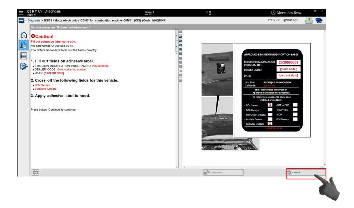
Complete the information on the APPROVED EMISSION MODIFICATION LABEL and attach it to the hood near the hood lock.
