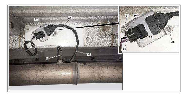
Install new NOx sensor control unit downstream of the SCR catalytic converter (27).
