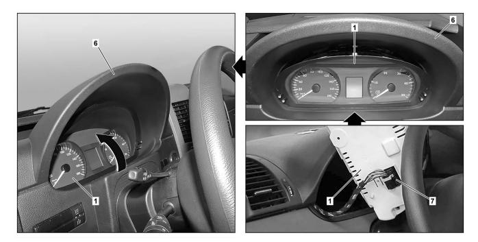
17 Put the new instrument cluster (1) in position and connect the electrical plug connection (7).
