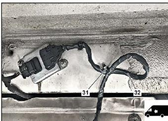
Install new NO<sub>X</sub> sensor control unit downstream of the SCR catalytic converter (4).
