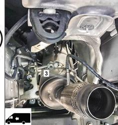
Clean the threads and the contact surfaces on the exhaust pipe.
