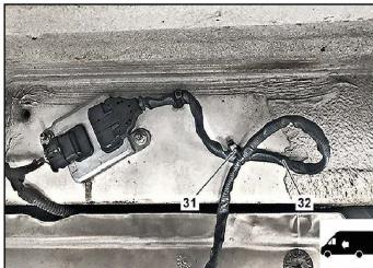
Install new NO<sub>X</sub> sensor control unit downstream of the SCR catalytic converter (4).
