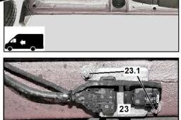
18 Disconnect the electrical plug connection (24) NOx sensor control unit upstream of the SCR catalytic converter (23).
