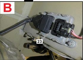
17 <u>Check</u> whether the NO<sub>x</sub> sensor control unit upstream of the SCR catalytic converter (23) is installed at location A or B.
