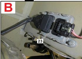
17 <u>Check</u> whether the NO<sub>x</sub> sensor control unit upstream of the SCR catalytic converter (23) is installed at location A or B.
