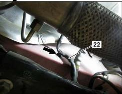
18 Disconnect the electrical plug connection (24) NOx sensor control unit upstream of the SCR catalytic converter (23).
