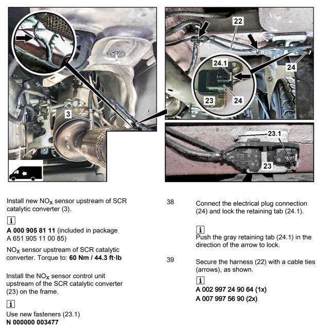
NO<sub>X</sub> sensor control unit. Torque to: **9 Nm / 6.6 ft·Ib**
