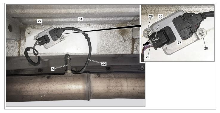
45 Install new NOx sensor control unit downstream of the SCR catalytic converter (27).
