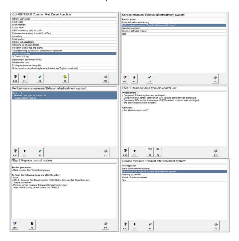
11. Replace the engine control unit (A 642 900 98 01).
