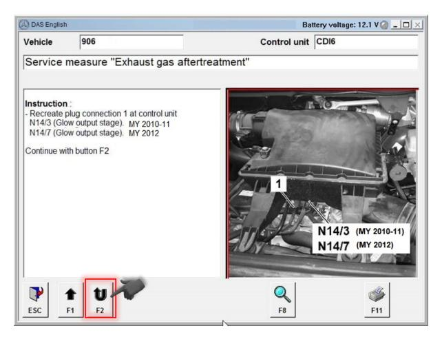
Connector 1 of glow output stage control unit (N14/3 on MY 2010-2011 or N14/7 on MY 2012) must be re-connected after CDI initial startup procedure.
