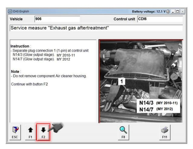
Connector 1 of glow output stage control unit (N14/3 on MY 2010-2011 or N14/7 on MY 2012) must be temporarily disconnected during the CDI initial startup procedure to help prevent pre-mature wear to steel glow plugs used on MY 2010-2012 Sprinter.
