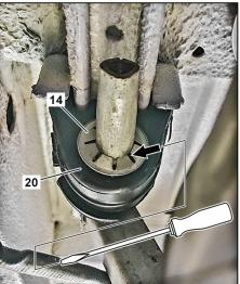
24 Remove and dispose the spring washer (14) on the holding bracket of the SCR catalytic converter (4).
