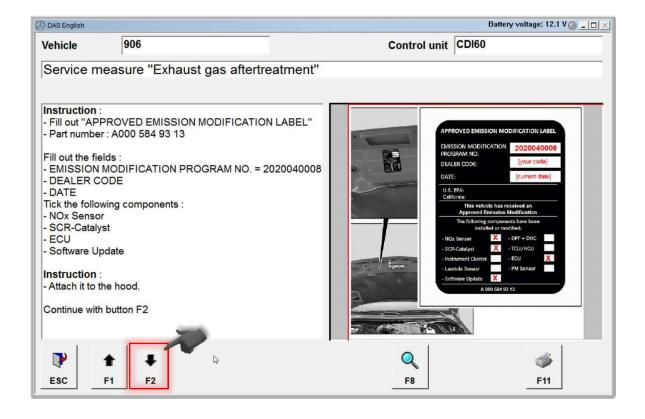
Complete the information on the APPROVED EMISSION MODIFICATION LABEL and attach it to the hood near the hood lock.
