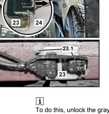
To do this, unlock the gray retaining tab (24.1) by moving towards the cable harness.
