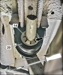
24 Remove and dispose the spring washer (14) 26 on the holding bracket of the SCR catalytic converter (4). i
