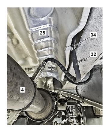
56 Postion new clamp (15) on the SCR catalytic converter (4).
