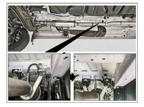
27 Loosen the clamp (15) at tailpipe (13) connection.
