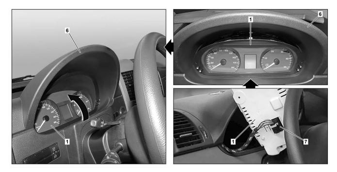
17 Put the new instrument cluster (1) in position and connect the electrical plug connection (7). **i**A 906 900 81 03 (mph)
