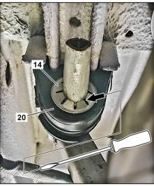
34 Remove and dispose the spring washer (14) 36 Remove the SCR catalytic converter (4). on the holding bracket of the SCR catalytic i converter (4). To do this, remove the SCR catalytic converter (4) from the decoupling i elements (20). This is done by bending up the individual
