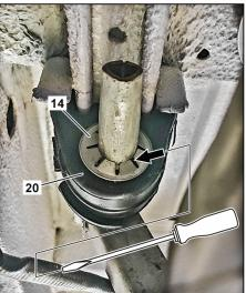
Remove and dispose the spring washer (14) on the holding bracket of the SCR catalytic converter (4).
