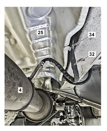
Postion new clamp (15) on the SCR catalytic converter (4).
