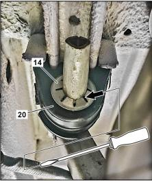
Remove and dispose the spring washer (14) on the holding bracket of the SCR catalytic converter (4).
