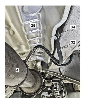
56 Postion new clamp (15) on the SCR catalytic converter (4). i
