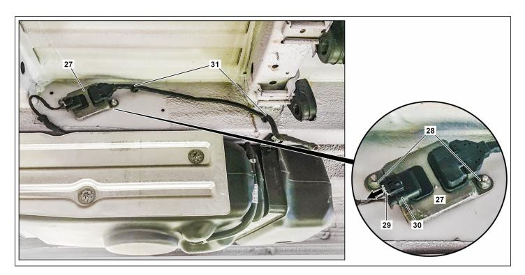
Disconnect the electrical plug connection (30) at the downstream  $NO_X$  sensor control unit (27).
