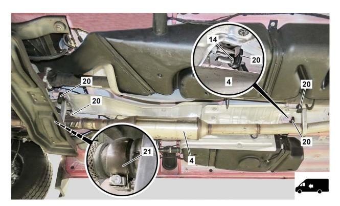
Position the new clamp (21) on the exhaust pipe.
