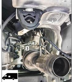
Clean the threads and the contact surfaces on the exhaust pipe.
