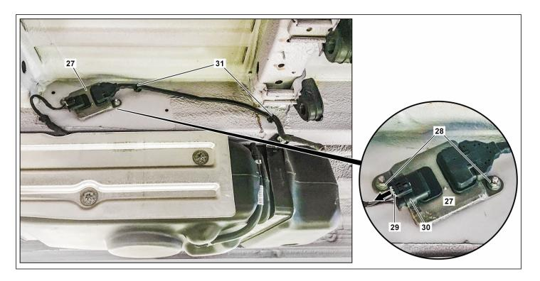
Disconnect the electrical plug connection (30) at the downstream NO<sub>X</sub> sensor control unit (27).
