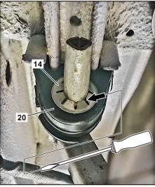
Remove and dispose the spring washer (14) 26 on the holding bracket of the SCR catalytic i converter (4). i elements (20). This is done by bending up the individual locking fins with a screwdriver. i i
