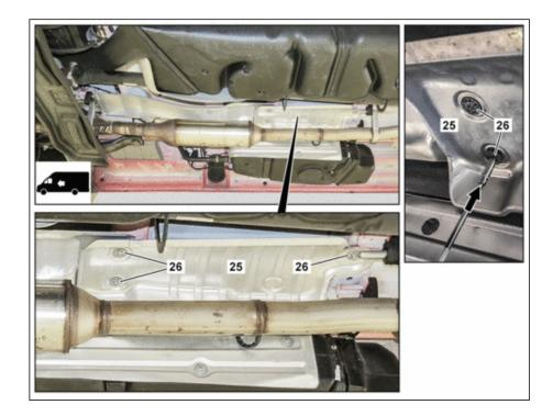
40 Install the new mounting tab (34) on the heat shield (25).
