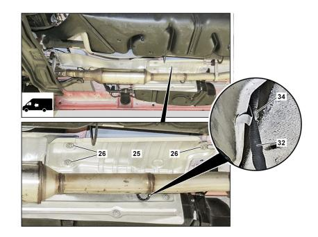
26 Remove the heat shield (25).
