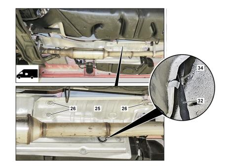
26 Remove the heat shield (25).
