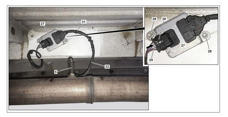
Install new NOx sensor control unit downstream of the SCR catalytic converter (27).
