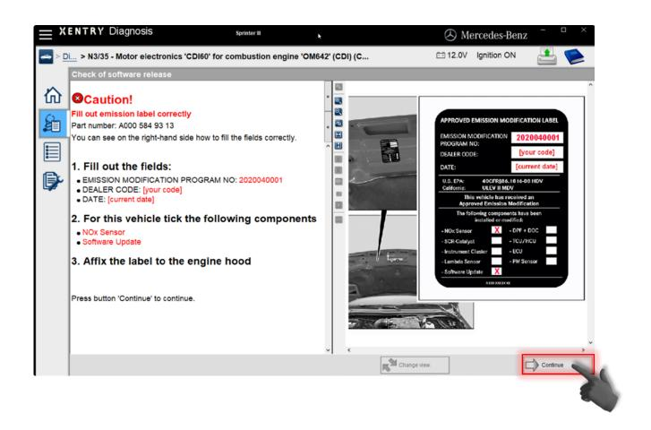
Complete the information on the APPROVED EMISSION MODIFICATION LABEL and attach it to the hood near the hood lock.
