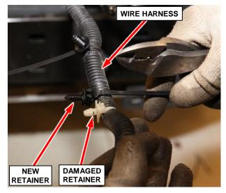
Figure 11 – Wire Harness Retainers
