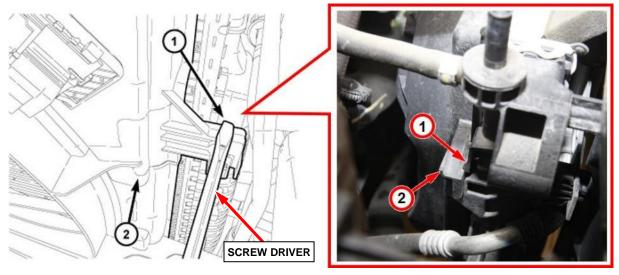
Figure 21 – Cooling Fan Module Mount Retaining Clip
