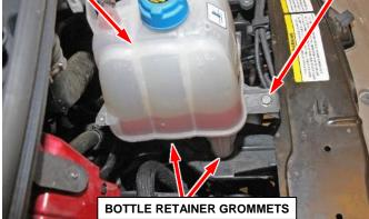
Figure 2 – Coolant Recovery Bottle
