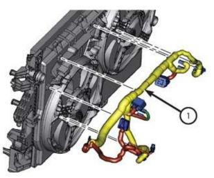
Figure 7 – Wire Harness Retainers
