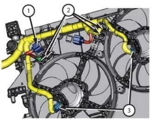
Figure 6 – Wire Harness Connectors
