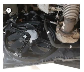
Figure 10 – Cooling Fan Module
