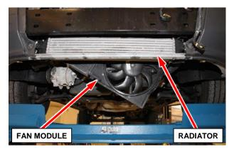
Figure 22 – Cooling Fan Module
