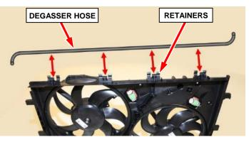
Figure 4 – Coolant Degasser Hose
