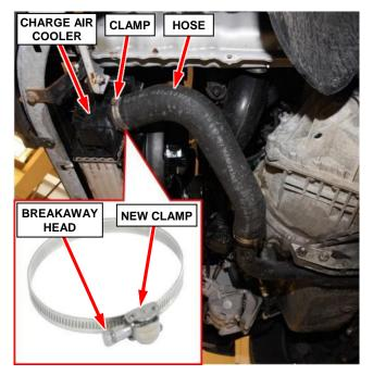
Figure 20 – Charge Air Cooler Hose
