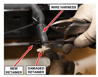
Figure 23 – Wire Harness Retainers
