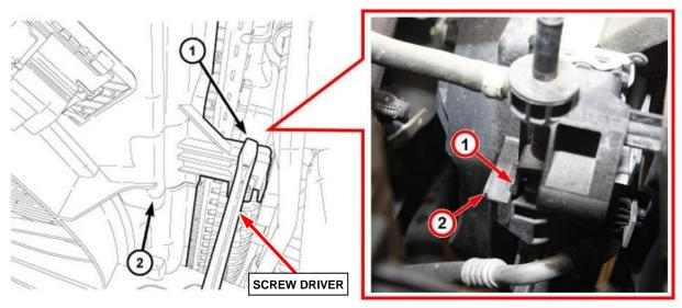
Figure 9 – Cooling Fan Module Mount Retaining Clip
