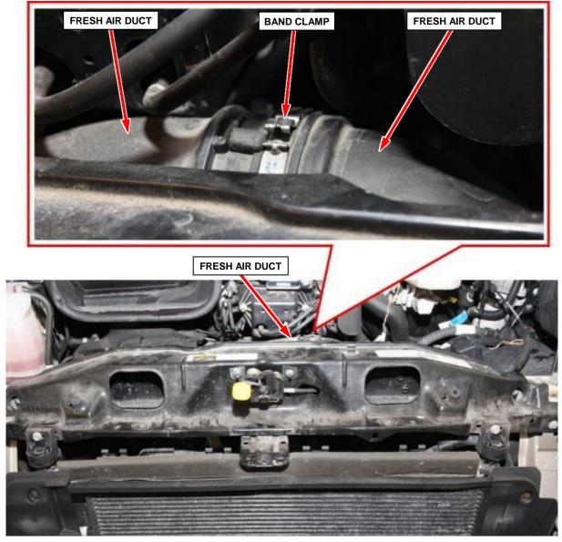
Figure 14 – Fresh Air Duct Band Clamp
