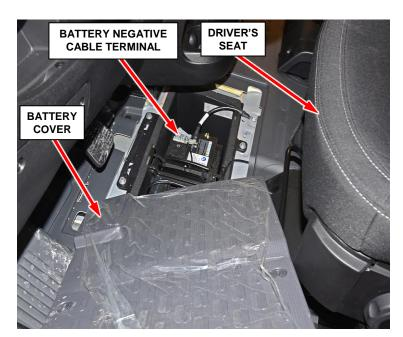
Figure 1 – Battery Cover and Negative Cable
