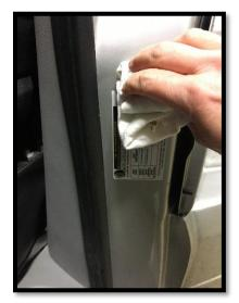
**<u>Step 3</u>**: Remove the corrected "Tire and Loading Infomormation" label and place it over the existing label on the on the Driver's Side B-Pillar.
