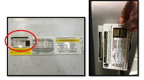
**<u>Step 4</u>**: Remove the corrected "Motor Home Occupant Cargo Carrying Capacity" label and place it over the existing label on the Passenger Side Door.
