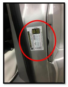
**<u>Step 2</u>**: Wipe directly over the existing labels with the denatured alcohol to clean the area.
