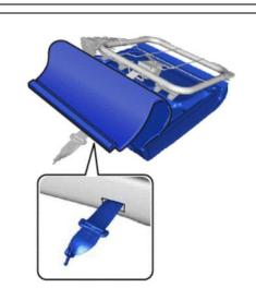
e. Engage the claws to install the 2 outer headrest supports.
