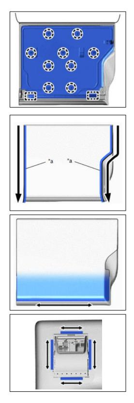
g. Engage the guides and claws to install the rear seatback board RH.
