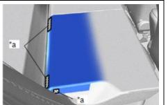
p. Engage the hook and loop fasteners.
