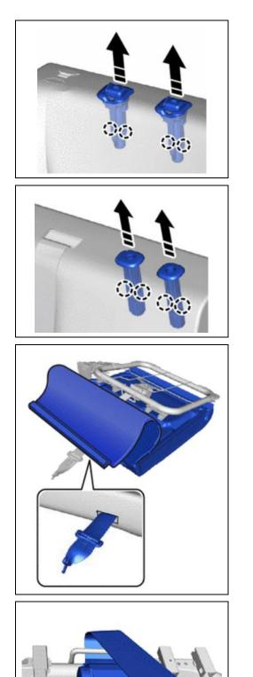
m. Disengage the claws to remove the outer headrest supports.
