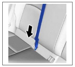
q. Connect the rear center seat belt to the lower buckle.
