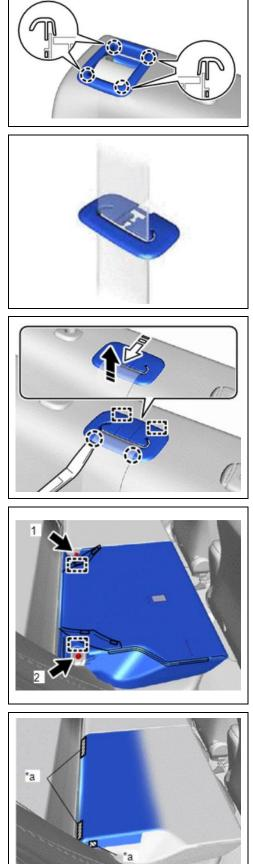
k. Engage the claws of the **NEW** seatback lock bezel.
