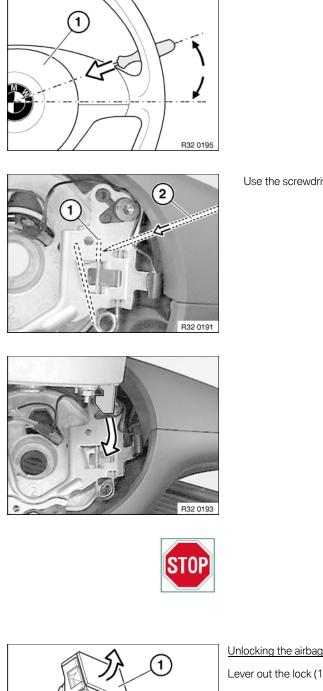
Insert a screwdriver through the opening on the rear side of the steering wheel and press on the lock. In the event of a spring resistance, press the lock up to the limit position and simultaneously pull away the airbag unit (1) from the steering wheel.
