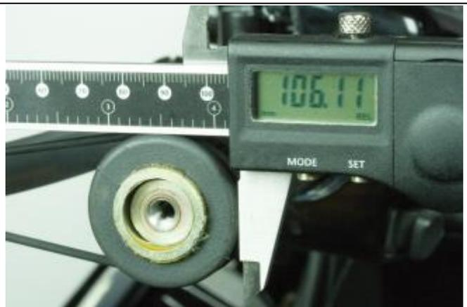
**IMPORTANT:** If the distance measured is not correct, repeat the entire bleeding procedure from the start.
