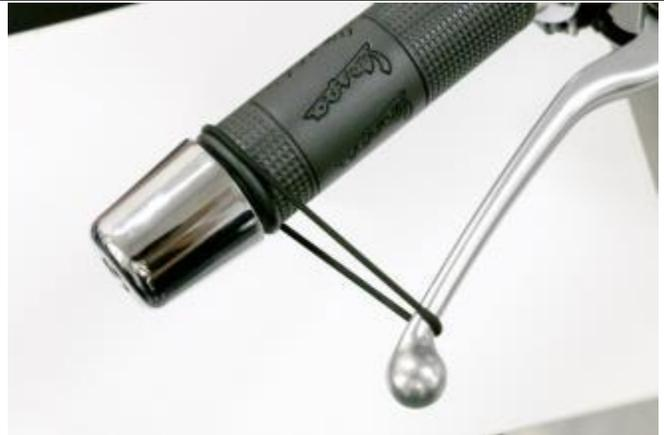
Place one end of the caliper gauge on the end of the hand grip as shown in the photo.
