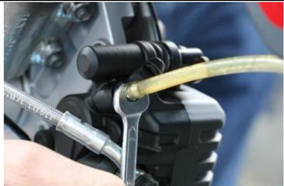
Check if the fluid contains air bubbles. Repeat the sequence described above **until only brake fluid containing no air bubbles is bled from the nipple for at least three consecutive check cycles.**
