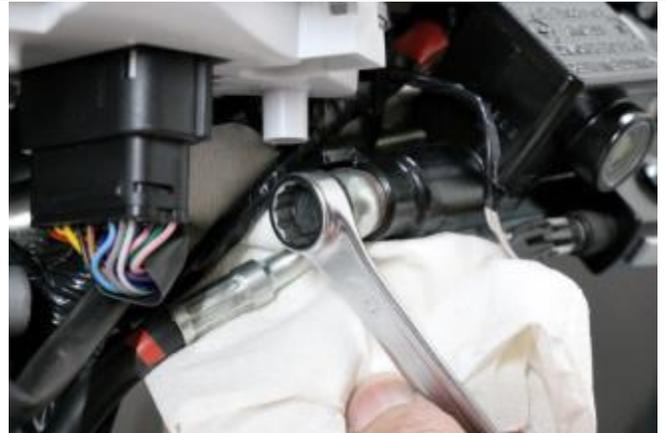
Fit the bleeding kit fitting with bleed nipple, P/N **AP8133945** with new copper washers, P/N **AP8113004**, and loosen the bleed nipple nut to open.
