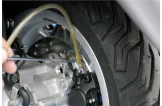
Check if the fluid contains air bubbles. Repeat the sequence described above until **only brake fluid containing no air bubbles is bled from the nipple for at least three consecutive check cycles.**
