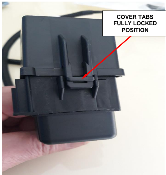
Figure 10 – Housing Cover Installed
