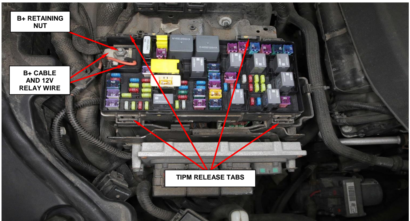
Figure 3 – TIPM Release Tabs
